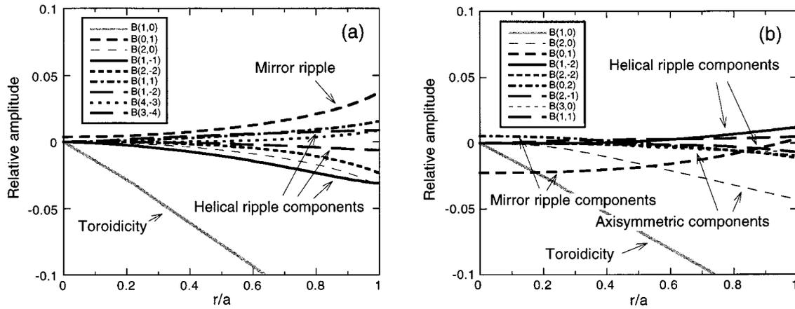
**Figure 2.** Boozer spectrum of magnetic field ripple components for (a) the 2b32 configuration and (b) the 2a36 configuration.  $B(m, n)$  ( $m$ , poloidal mode number;  $n$ , toroidal mode number) is the amplitude relative to that of the toroidal field.
