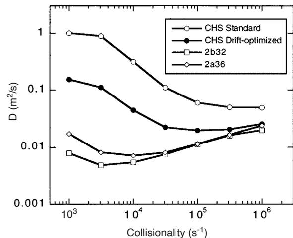
**Figure 3.** Neoclassical diffusion coefficients for CHS and CHS-qa. The electric field is not included.
