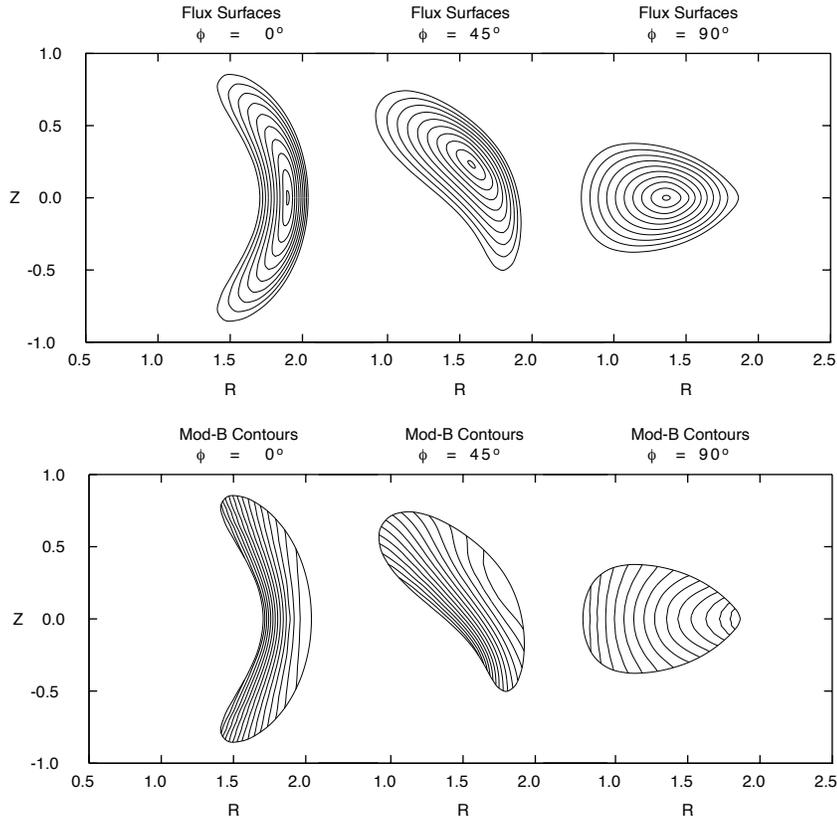
**Figure 1.** Magnetic surfaces and contours of magnetic field strength for the 2b32 configuration, for 3% average beta equilibrium.
