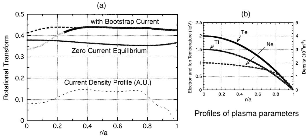
**Figure 4.** (a) Rotational transform profile with self-consistent bootstrap current. The current density profile is shown in arbitrary units. The rotational transform of the equilibrium with the assumption of zero average current is also shown for comparison. (b) Plasma profiles used in the calculation.
