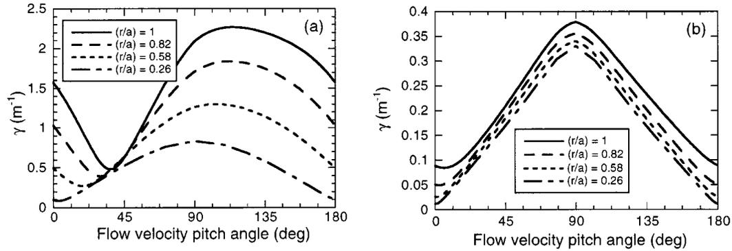
**Figure 5.** Comparison of magnetic field variation  $\gamma$  for (a) CHS and (b) CHS-qa (the 2b32 configuration).  $\gamma$  is calculated for four selected magnetic surfaces. As for the flow velocity pitch angle,  $0^\circ$  corresponds approximately to the toroidal direction and  $90^\circ$  to the poloidal direction.
