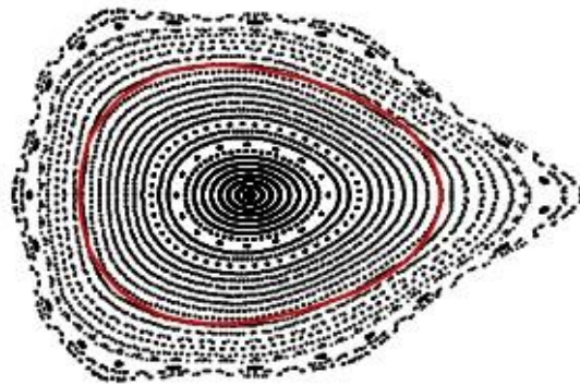
Fig. 4.3.6-2 Punctual plots of magnetic surfaces for CFQS configuration produced by 16 modular coils. Red line corresponds to the LCMS of the 3rd plot in Fig. 4.3.6-1
